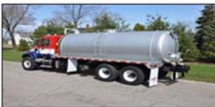
A temporary water and pumping truck are all the equipment the Titan Process requires to service oil fields. The trucks are rented and standard oil industry equipment. The nutrients are shipped to the site, mixed with water and injected into the existing water system at the field. The Process is applied every 3-4 months.
